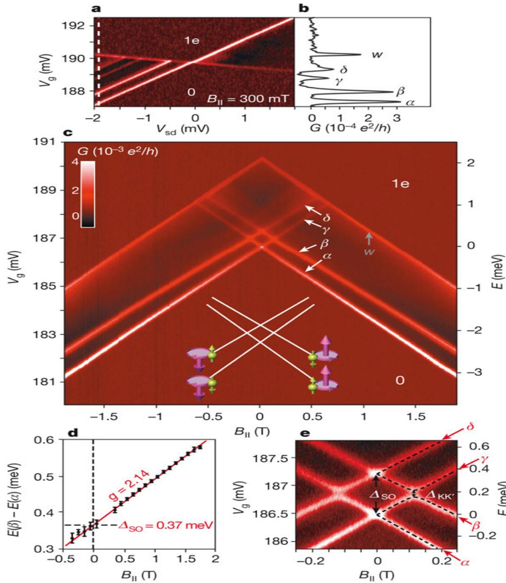
Direct measurement of single-particle levels via finite-bias cuts in Coulomb Blockade spectroscopy
