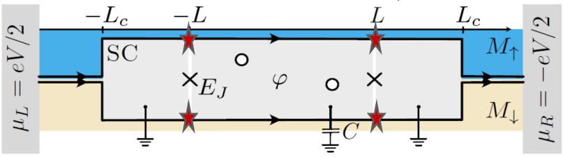
Add central floating superconducting (SC) island to Majorana interferometer & measure AC conductance between metallic leads
