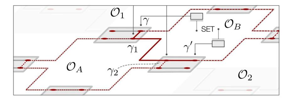
Read out of stabilizers: tunnel conductance via attached leads, noninvasive (no plaquette flip) measurement Controlled plaquette flip: Transfer 1 electron through code by changing gate voltages on attached pair of SETs
